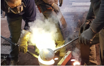
Pouring the bronze into the mould
