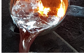
Detail of bronze cast at 1200/1300 degrees
