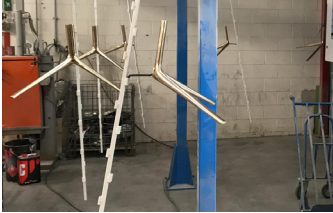
Preparing the legs for varnishing
